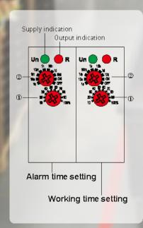
Please rotate ② to set timming, and rotate ① to set the timming percentage.
